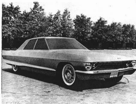
Above, full size clay model of XP-727 #2, an Eldorado forecast, 1961. Below, a four-door exercise, XP-727 #3, highly finished, 1962.
