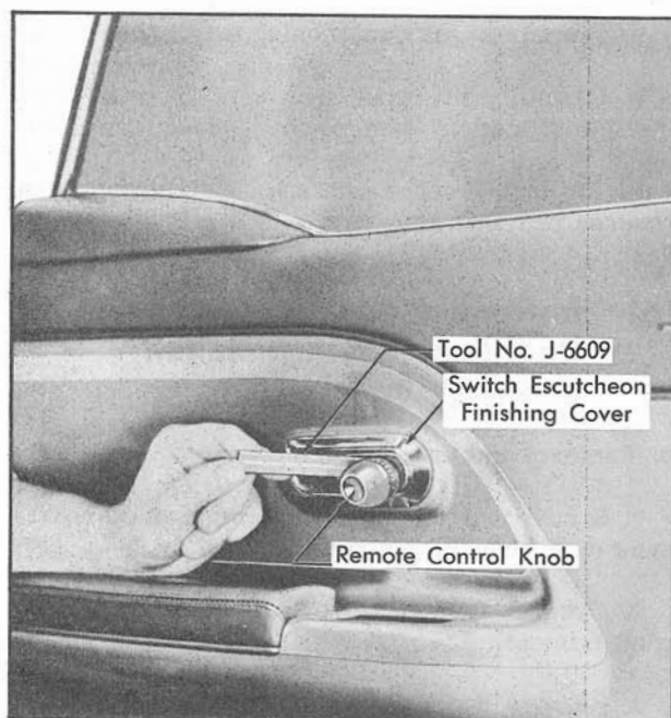
Fig. 17-11 Remote Control Knob Removal
