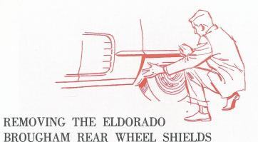
There are three hooks attaching the rear wheel shields to the car fender. The forward hook is operated with one lever, and the center and rear hooks are operated with the rear lever. Push these levers toward the wheel and pull down to disengage the hooks. Tip the shield outward at the top while raising up and away from the mounting hooks.
