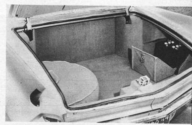
The entire trunk of the Eldorado Brougham is covered with a nylon frieze material, including the decklid, the spare tire (laid horizontally) and the fold-down cover over the battery. Though the trunk is not as great in cubic space as some cars, it still holds ample luggage.
