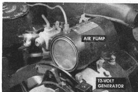
AIR PUMP mounted on top of the car's generator provides air for the air-suspension system. Its operation is automatically controlled by three levelizers and a master control.
