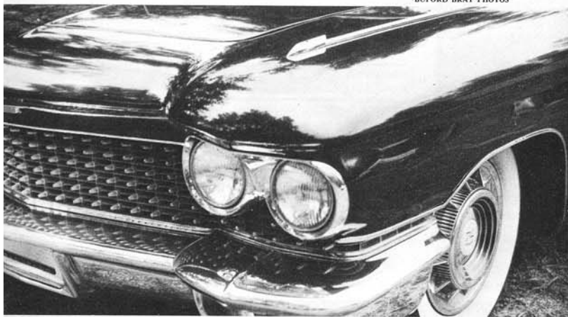
Italian craftsmen hammered out Eldorado's body panels by hand in Pinin Farina's shops. The cars were then assembled on stationary lines.
