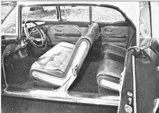
Brougham's doors automatically lock in 14-inch posts when shut. Car has no central body pillars.
