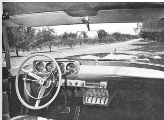
Conti's dash is much simpler than Eldo's, in fact seems spartan, yet includes all gauges and tach.
