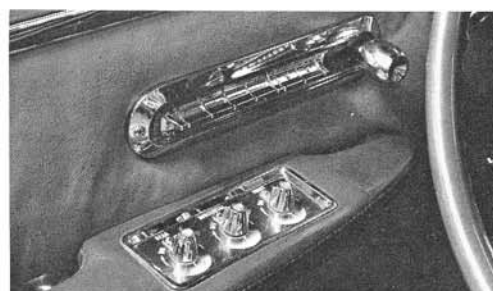
Door controls include 6-way "memory" power seat, buttons for door locks, electric windows.
