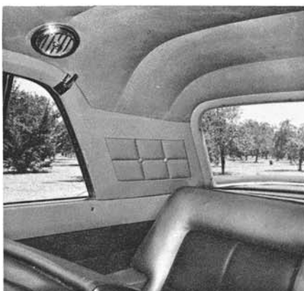
Mark II has 4 roof registers for air conditioning. Passengers tend to complain of cold heads.
