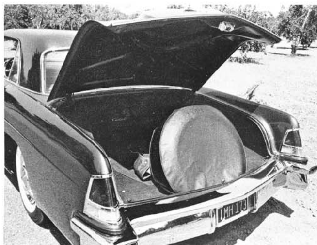
Mark II's trunk is blocked by spare, which also cuts severely into space. Perhaps if tire cantilevered backwards like Zephyr's, it'd be handier.
