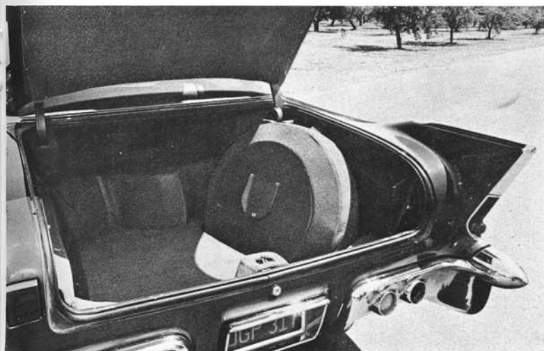
Brougham's trunklid raises and lowers with electric motor, is activated by button in glovebox or key. If battery goes dead, no access to trunk.
