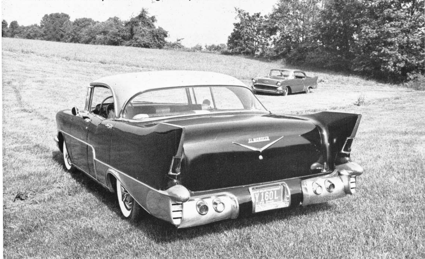
Eldorado Brougham illusion is especially convincing from rear. Fiberglass fins use 1956 Plymouth lenses, and bumper bullets come from '54 Mercury.
