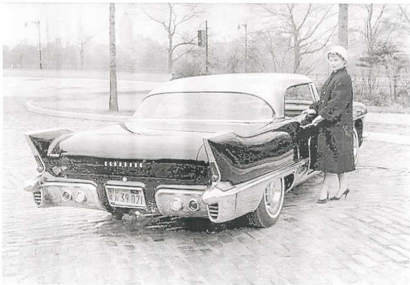
THE CADILLAC ELDORADO BROUGHAM -- This super luxury sedan features dramatically styled rear quarter panels and swept back tail fin styling with delicately formed stainless steel fender skirts extending from the vertical molding to the rear bumper section. Protective chrome rear bumper pieces in three sections are mounted flush with the body.
