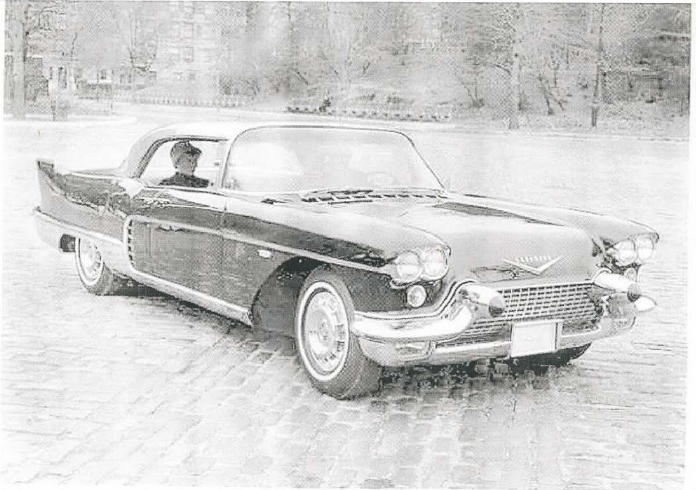
THE CADILLAC ELDORADO BROUGHAM -- This is the exclusive Cadillac Eldorado Brougham. An ultra luxury four-door model, the Brougham features such outstanding engineering advances as the four headlamp system, air suspension and tubular center X-frame. The Brougham stands 55-1/2 inches high and is 216.3 inches long.
