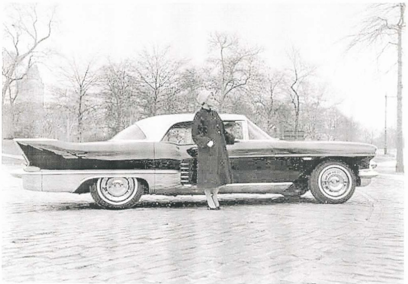
THE CADILLAC ELDORADO BROUGHAM -- The stainless steel roof and stainless steel moldings in contrast with the dark exterior of Cadillac's Eldorado Brougham present a new appearance in sculptured metal. The doors on the Brougham open outward from a center locking plate. The rear doors are secured to this plate when the car is in any drive gear.
