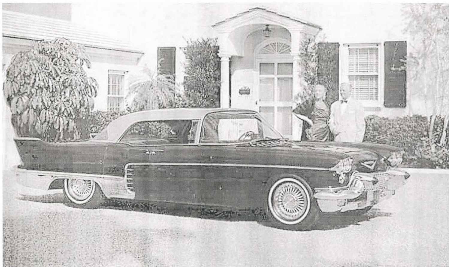
Sweeping surfaces of lustrous stainless steel—used for the entire roof and for the rear fender skirts—provide the distinctive 1957 Cadillac Eldorado Brougham with sleek, long-lasting beauty.
